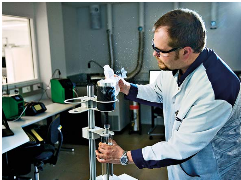
Toni Alatalo, Calibration Engineer, preparing the triple point of water.
